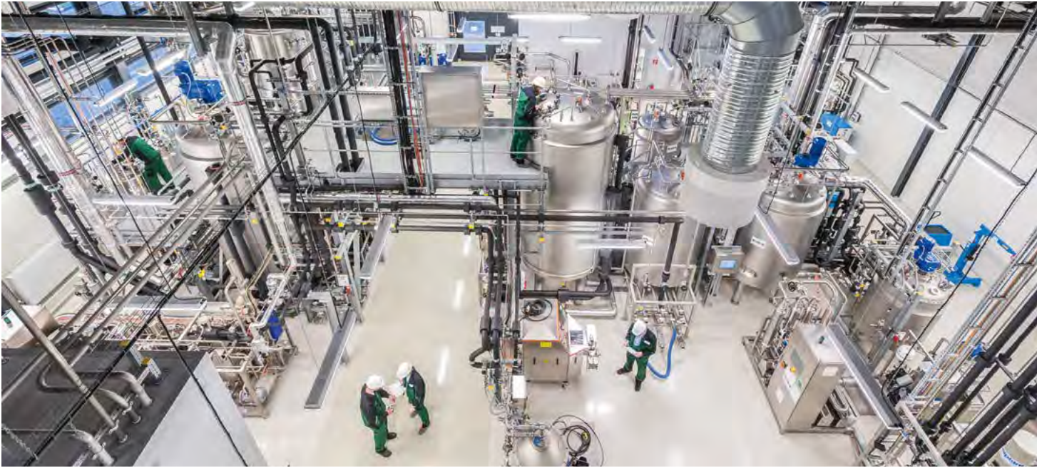
Biotechnology module consisting of plants for cultivating microorganisms and product processing
