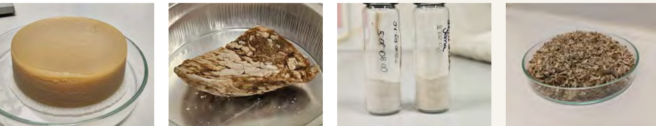
From left to right: precipitated pectin, dried pectin, ground pectin, raw material – sugar beet after sugar extraction
