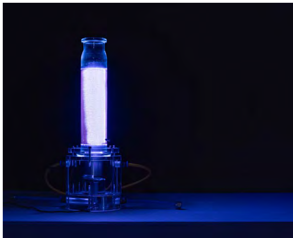
Plasma reactor for purifying water on a laboratory scale
