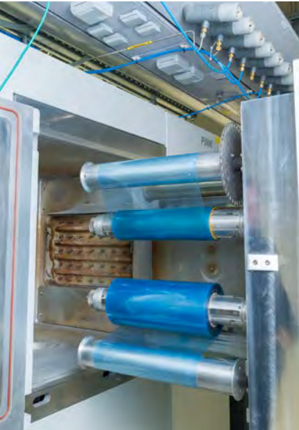
Continuous finishing with a PFAS-free non-stick layer in the roll-to-roll process
