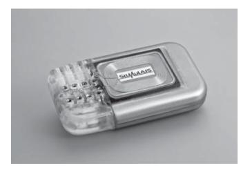
The implant uses electrical pulses to stimulate muscles. In the future, the unit will be implanted in the patient's groin area. The picture shows the prototype of the implant. (© Fraunhofer IPMS) | Picture in color and printing quality: www.fraunhofer.de/press
