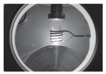
The researchers rely on the melt spinning process for the recycling of permanent magnets. For this, the material is melted in a crucible using an induction coil and subsequently poured onto a copper wheel. (© Fraunhofer Project Group IWKS) | Picture in color and printing quality: www. fraunhofer.de/press
