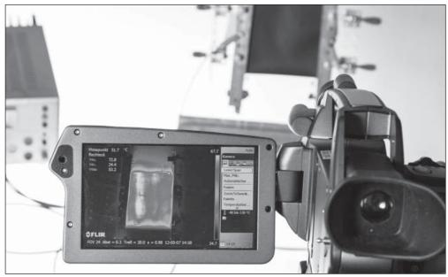
In order to analyze the heating effect of the films for cars, the researchers connected them to a power source and monitored them using a thermo camera. (© Fraunhofer IPA) | Picture in color and printing quality: www.fraunhofer.de/press
