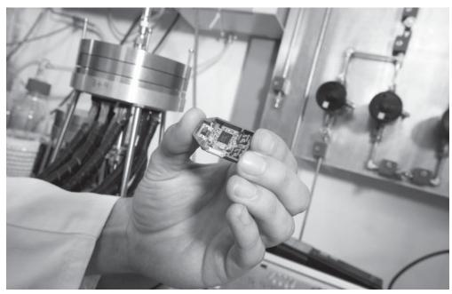
In Fraunhofer IPM's sensor, dyes react to gases – and trigger an alarm, even in the case of smoldering fires. (© K.-U. Wudtke/Fraunhofer IPM) | Picture in color and printing quality: www.fraunhofer. de/press
