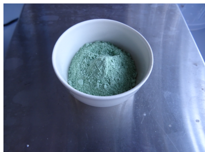
Precursor of a copper-based catalyst synthesized at the Straubing branch of the institute. (© Fraunhofer IGB)
