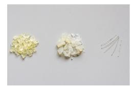
From wood waste to high-performance polymers: Terpenes from turpentine oil are converted to biobased, heat-stable polyamides. (© Fraunhofer IGB) | Picture in color and printing quality: www.igb.fraunhofer.de/press PRESS RELEASE October 9, 2019 || Page 3 | 3
