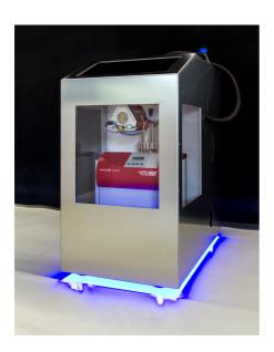
With this compact mass spectrometer up to 30 components can be analyzed simultaneously in the gas phase and a liquid.
