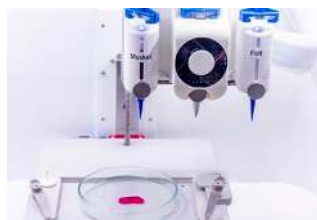
Cultivated meat is produced using a 3D printing process.
