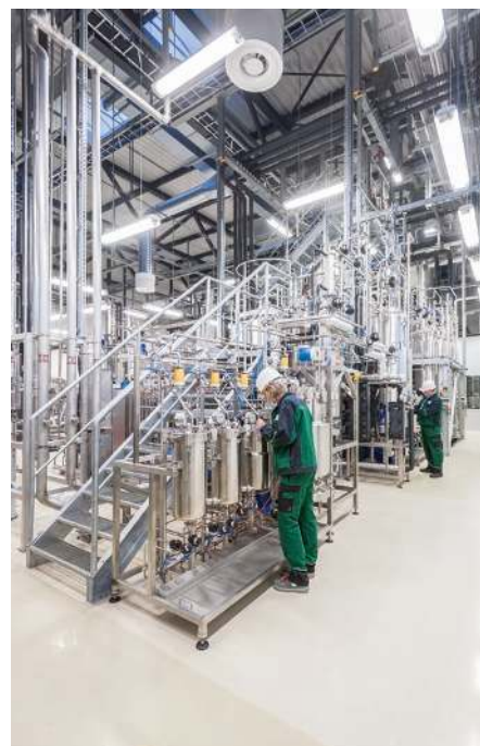
Bioreactor cascade for scaling fermentation processes at Fraunhofer CBP
