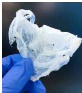
The biodegradable plastic polyhydroxyalkanoate (PHA), produced from organic acids
