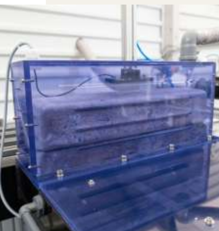
Left: ePhos®: encased magnesium ingot as sacrificial anode
