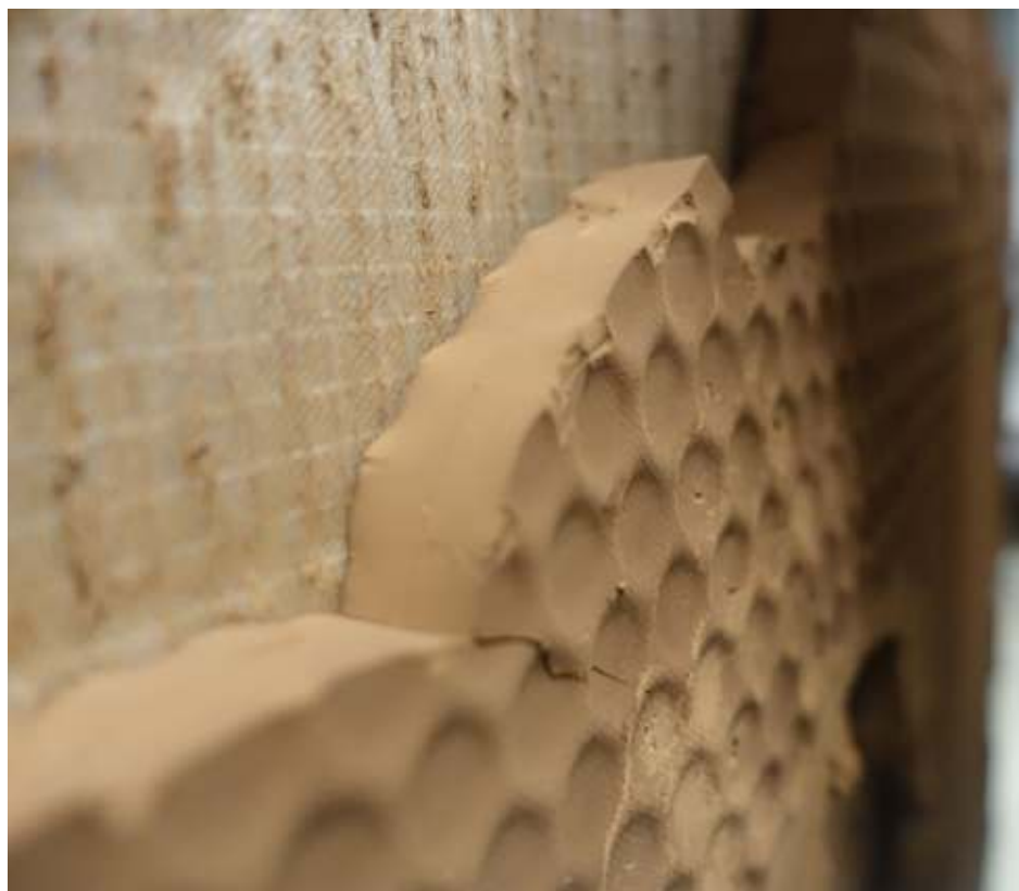
Lignin separation by filter press at Fraunhofer CBP
