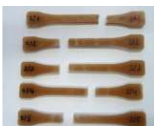
Hydrophobic cellulose in the drop test (top left), comminuted cellulose fibers (cutting mill, top right) and fracture pattern of test rods 1BA (fiber content ten percent, left)
