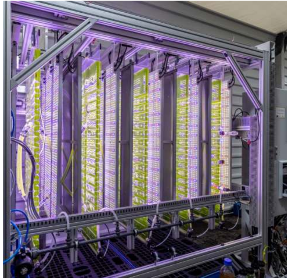
Microalgae in a novel photobioreactor system bind \text{CO}_2 and produce a plant-strengthening biomass.
