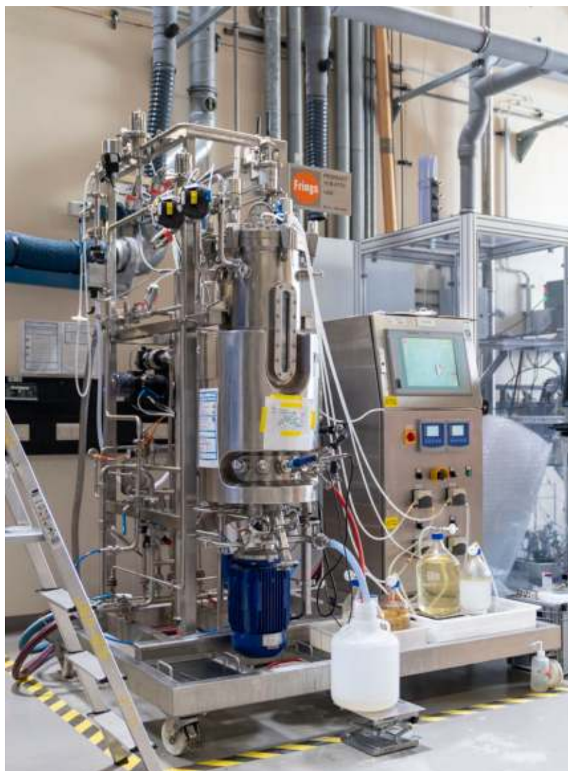
Closed 50-liter stainless steel bioreactor for cultivating purple bacteria on a larger scale
