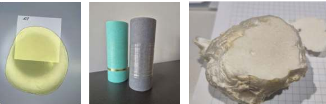
Further processing of the caramides into cast polyamide sheets (left), fibers (mono-filaments, center) or foams (right) to demonstrate various applications
