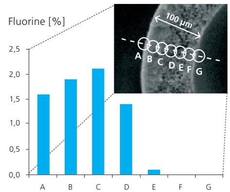
**Figure 3:** Distribution of chemical functionality over the cross section of a hollow fiber following derivatization of the surface-bound amino groups with pentafluorophenylalanine, analysis by ESCA.
