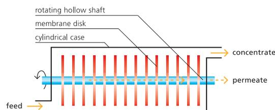
Figure 2: The rotating disk filter developed at the Fraunhofer IGB for use in preliminary filtration as well as in membrane bioreactors.
