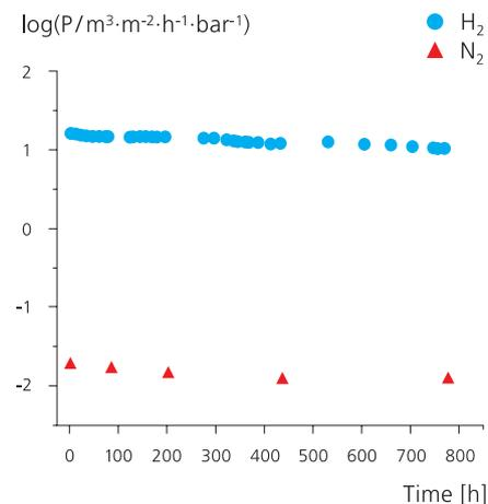
Figure 2: Hydrogen permeability and selectivity of Pd-coated  $\text{Al}_2\text{O}_3$  capillaries at 430 °C.
