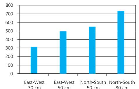
**Figure 2:** Biomass productivity levels of *Phaeodactylum tricornutum* in June under outdoor conditions with different reactor orientations and distances.
