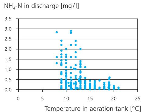
**Figure 1:** Levels of ammonium nitrogen in the discharge from a treatment plant as a function of the temperature in the aeration tank.
