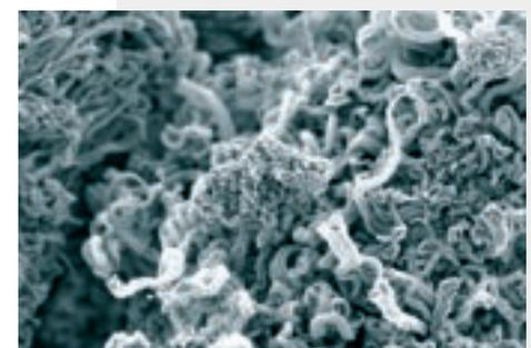
**Figure 2:** Scanning electron microscopy images of different raw materials composed of multi-wall carbon nanotubes (MWNT). The images clearly show the differences in quality in terms of their macroscopic structure.
