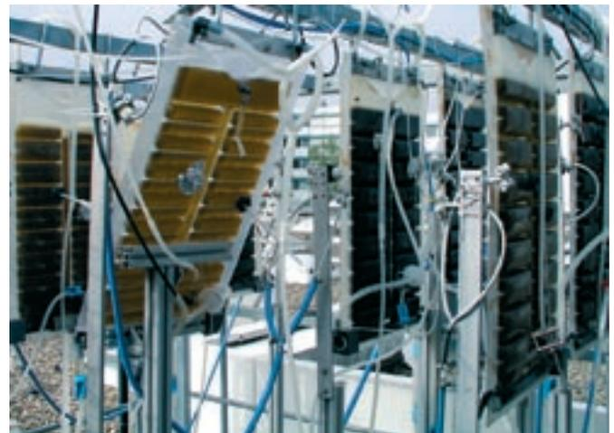
**Figure 4:** FPA reactors at the outdoor production plant on the Institute Site in Stuttgart.
