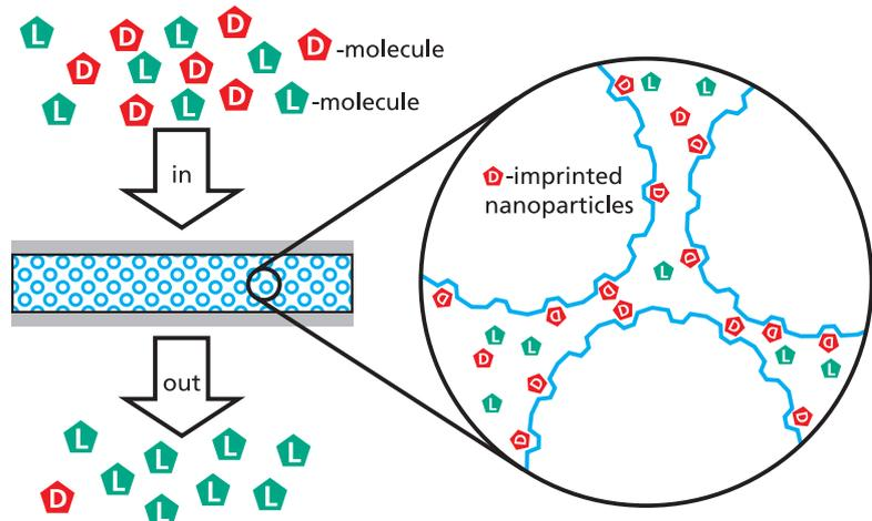
Figure 3: Schematic construction and functioning of a composite membrane with molecularly imprinted polymer particles.
