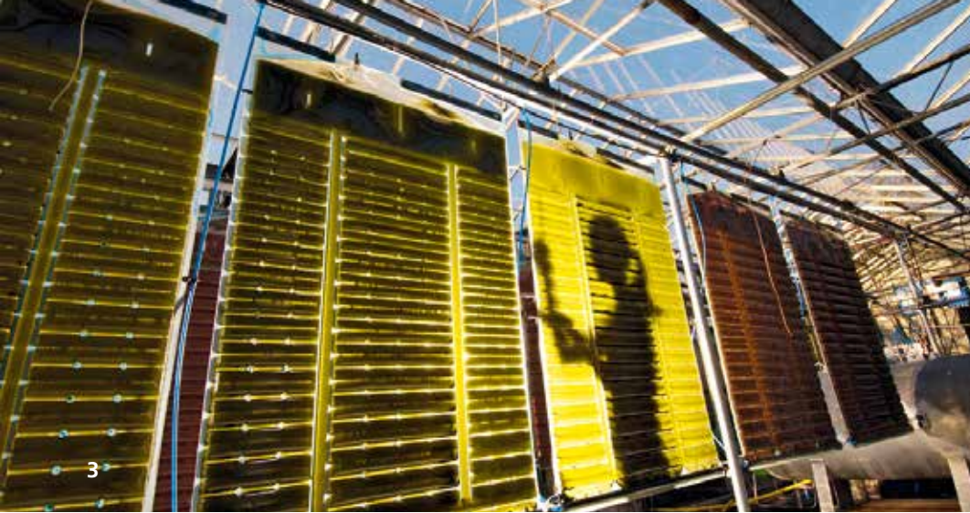
3 Pilot plant with 180-liter photobioreactors for culturing algae
