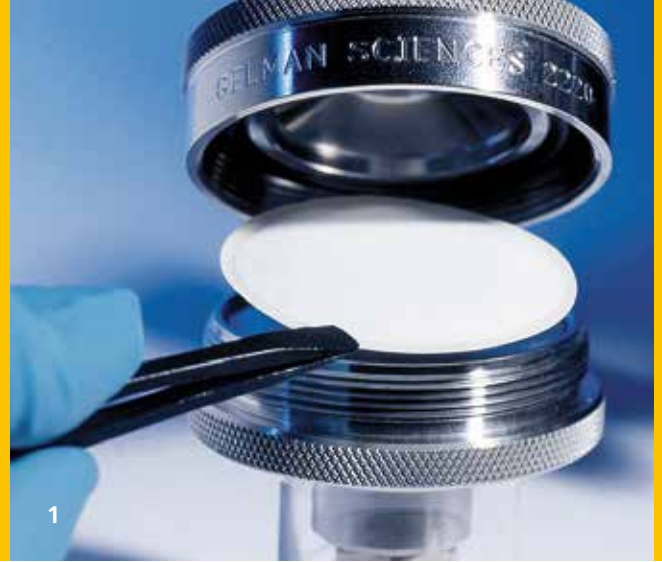
1 Composite membrane with functionalized nanoparticles to enable selective separation processes
