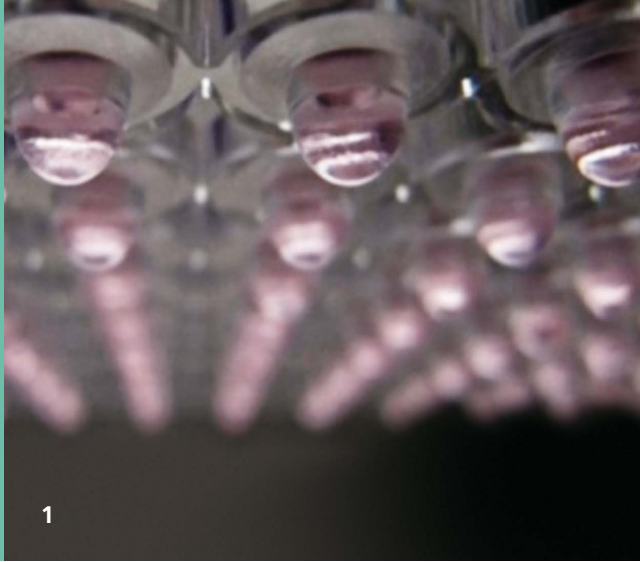
1 Automated hanging-drop (HD) cell culture using special HD plates.
