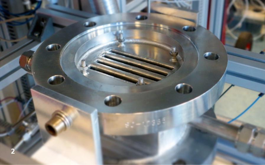
2 Reactor for producing long-chain alcohols using the Fischer-Tropsch process.
