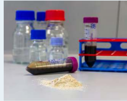
top: Struvite recovered from wastewater can be used as a N and P slow-release fertilizer
