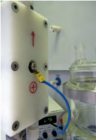
Laboratory cell for anodic oxidation and cathodic reduction.
