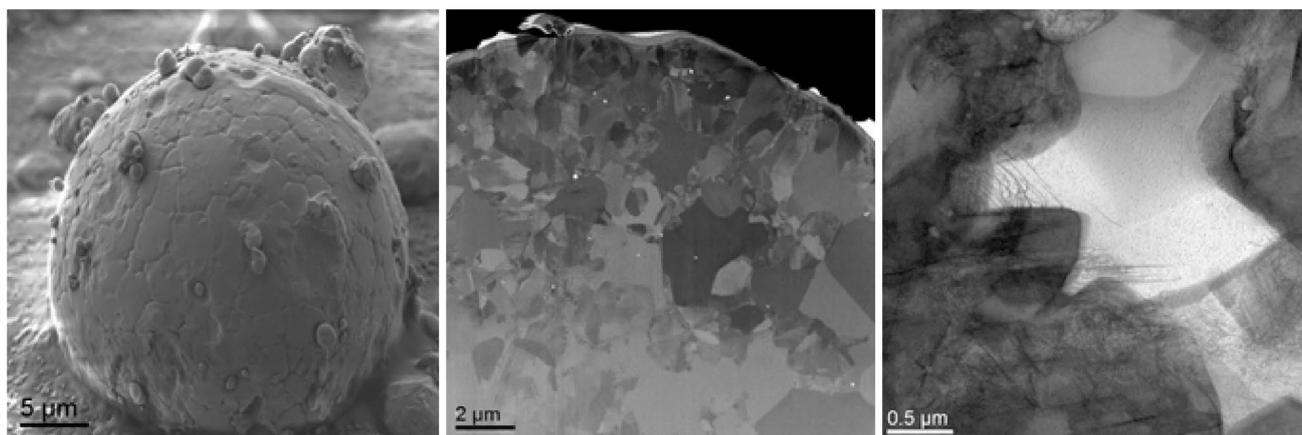
**Fig. 6** Investigation of surface structure (left), internal structure (center) and lattice defects (right) in combination of scanning electron microscopy (SEM), focused ion beam (FIB) and transmission electron microscopy (TEM)
