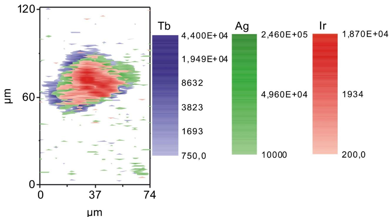
**Fig. 5** Analysis of silver nanoparticle distribution in individual cells by spatially resolved bio-imaging using laser ablation inductively coupled plasma mass spectrometry (LA-ICP-MS)
