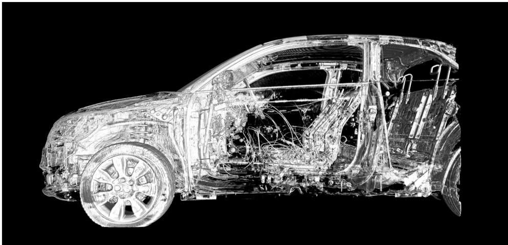
Through the eye of the XXL CT scanner: A car reveals its innermost secrets at the Fraunhofer Development Center for X-ray Technology EZRT in Fürth. (© Fraunhofer IIS) | Picture in color and printing quality: [www.fraunhofer.de/press](http://www.fraunhofer.de/press)
