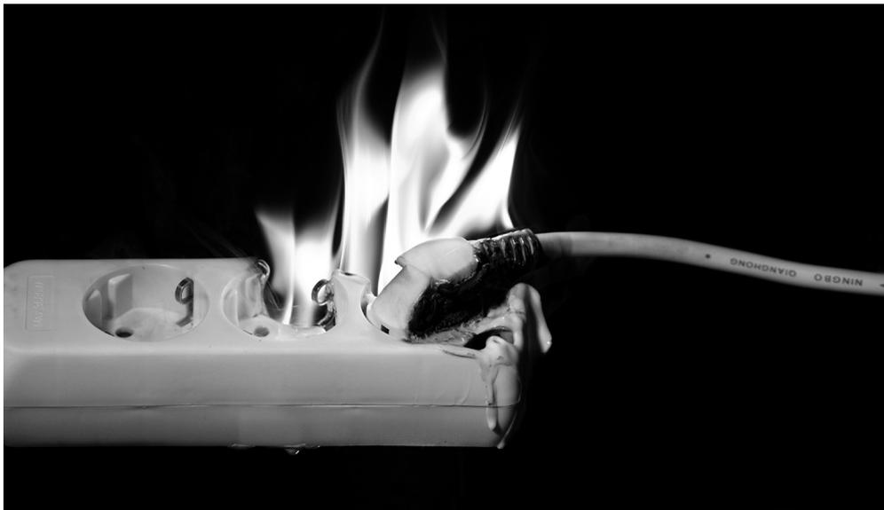
Many multi-plug connectors pose a fire risk, as they can overheat if the current flow is high. Flame retardants in the connector can prevent fires or slow the spread of the blaze. (© Fraunhofer LBF) | Picture in color and printing quality: [www.fraunhofer.de/press](http://www.fraunhofer.de/press)
