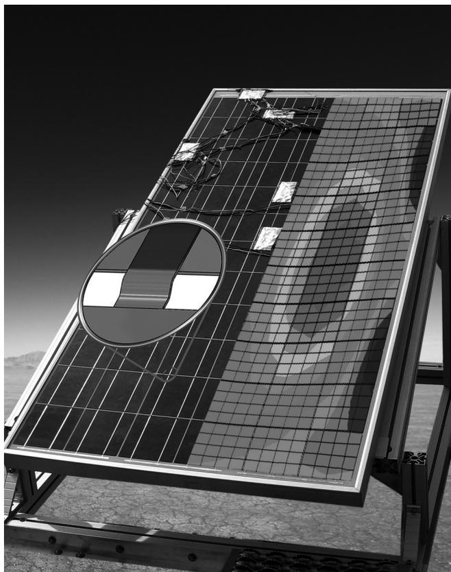
Sensors measure the elongations that arise in solar modules. Their operating life can be calculated from this data. (© Fraunhofer IWM) | Picture in color and printing quality: [www.fraunhofer.de/press](http://www.fraunhofer.de/press)
