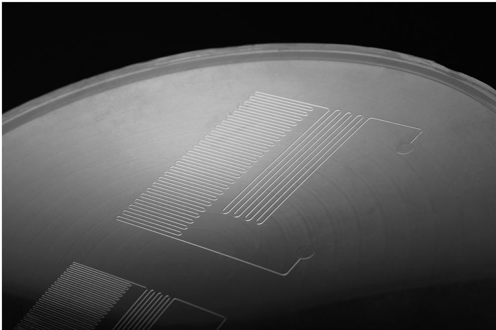
Microfluidic negative for structuring films. (© Fraunhofer IPT) | Picture in color and printing quality: [www.fraunhofer.de/press](http://www.fraunhofer.de/press)
