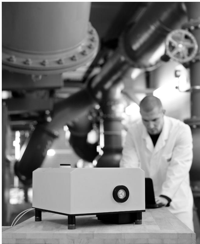
**Little larger than a shoebox, the demonstrator was developed as part of the IRLSENS project. It is a quick and automated way to analyze water samples at the waterworks itself. (© Martin Wagenhan/ Fraunhofer IAF) | Picture in color and printing quality: [www.fraunhofer.de/press](http://www.fraunhofer.de/press)**
