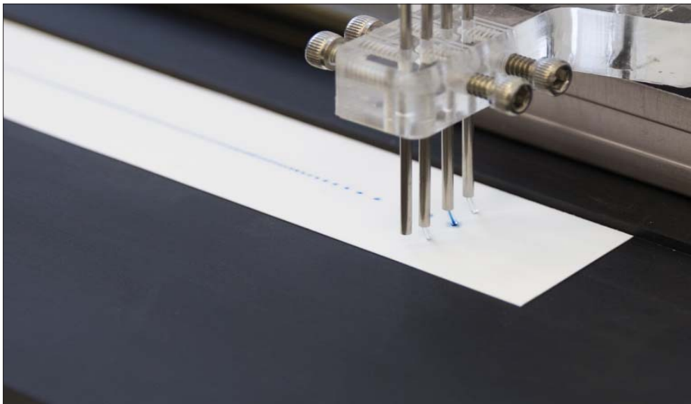
Production of ImmuStick: Application of immune receptors onto the test strip. © Fraunhofer IGB | Picture in color and printing quality: www.fraunhofer.de/en/press
