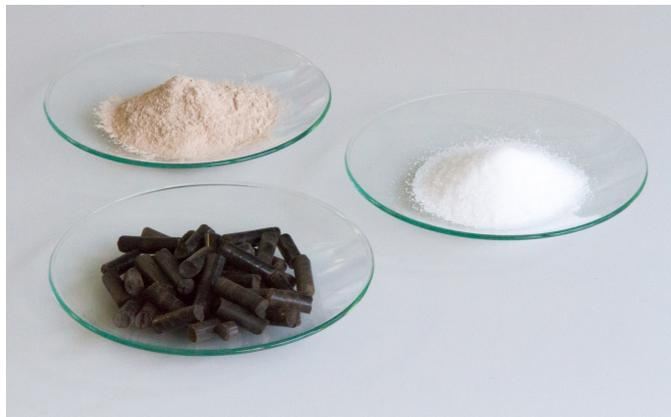
**With the BioEcoSim process, livestock manure can be converted into valuable phosphorus fertilizers (rear), nitrogen fertilizers (right) and soil conditioners (front). (© Fraunhofer IGB) | Picture in color and printing quality: [www.igb.fraunhofer.de/press](http://www.igb.fraunhofer.de/press)**
