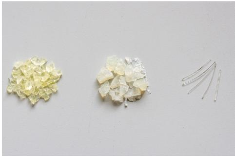
**From wood waste to high-performance polymers: Terpenes from turpentine oil are converted to biobased, heat-stable polyamides. (© Fraunhofer IGB) | Picture in color and printing quality: [www.igb.fraunhofer.de/press](http://www.igb.fraunhofer.de/press)**
