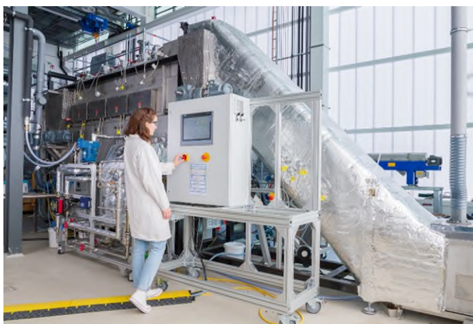
Fig. 1 Using electricity-generated superheated steam instead of hot air for industrial drying processes can drastically lower energy consumption. © Fraunhofer IGB
