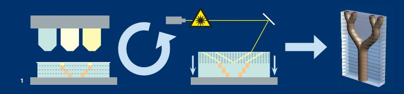
1 Scheme of the combined inkjet and TPP manufacturing process.
