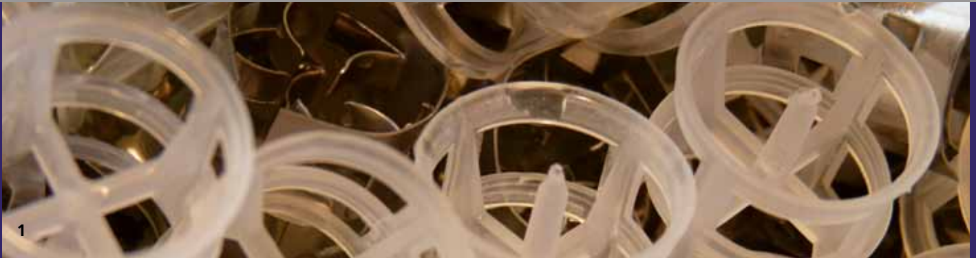
1 Packing materials coated with adsorber particles.
