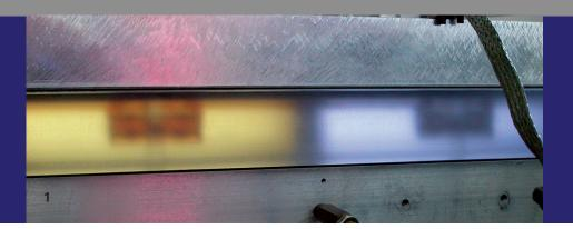
Plasma sterilization treatment of two Sterisafe®-sterile containers made of different materials
